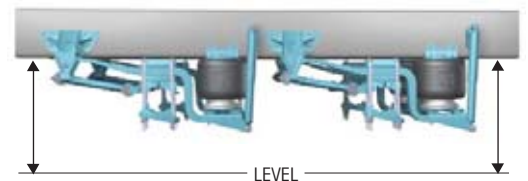
Proper vehicle ride height and level frame
