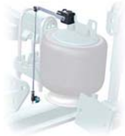
Height Control Valve
